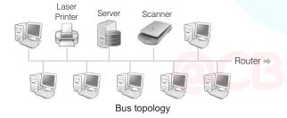
All the computers or devices are directly connected to the data line. The data is transmitted in small blocks known as packets. Each packet has a header containing the destination address.
